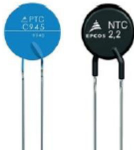
Gambar 2. Sensor Suhu NTC dan PTC (thermistor)
