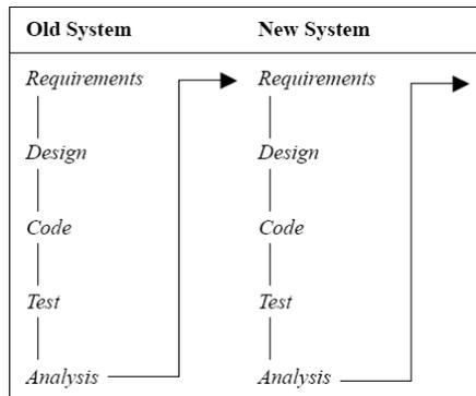
**Gambar 8.3 Iterative-Enhancement Model**
