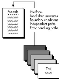
Gambar 7.6 Unit Testing
