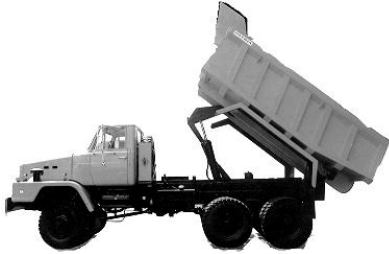
Gambar 24b. Dump Truck on road
