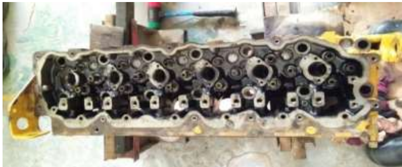
Gambar 2.3 cylinder head ohv
