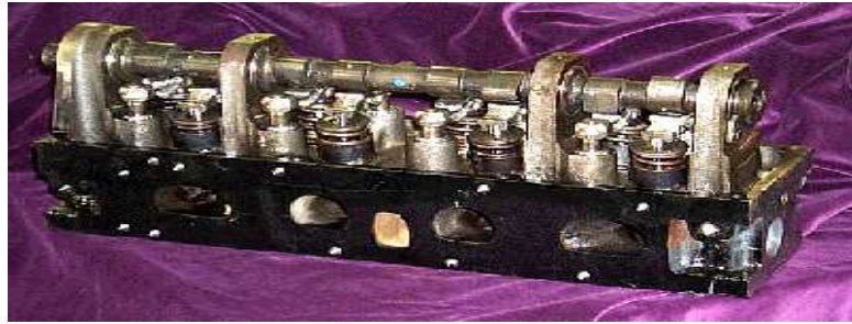
Gambar 2.4 cylinder head ohc (over head camshaft)
