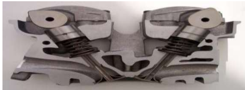
Gambar 2.5 cylinder head dohc (double over head camshaft)
