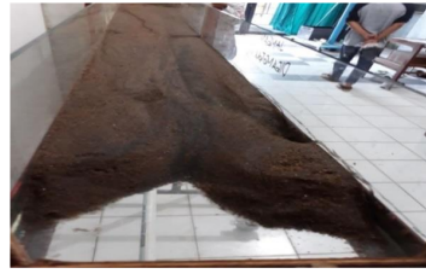
Figure 13. Erosion and Sedimentation Pattern on 90 Minute
