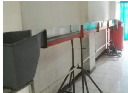
Figure 10. Open Channel Standard Flume
