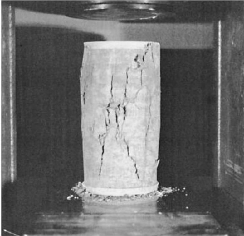
Figure 3-2 Typical failure mode of concrete in compression.
