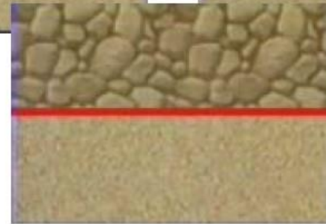
Separation with Geosynthetic
