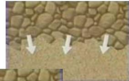
Aggregate Intrudes Subgrade
