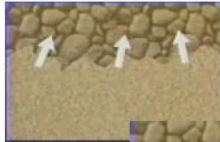
Soil Fines Pump into Aggregate
