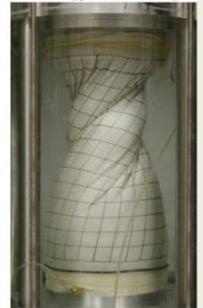
Photo 5. Deformation of specimen during undrained cyclic torsional shear test up to extremely large strain
