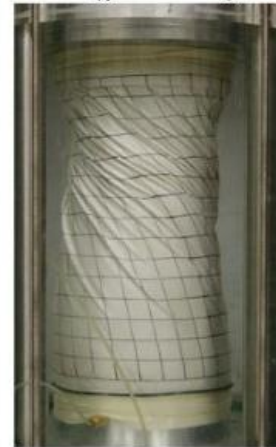
Photo 5. Deformation of specimen during undrained cyclic torsional shear test up to extremely large strain
