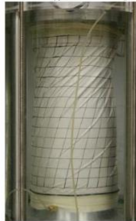
Photo 5. Deformation of specimen during undrained cyclic torsional shear test up to extremely large strain
