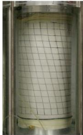
Photo 5. Deformation of specimen during undrained cyclic torsional shear test up to extremely large strain
