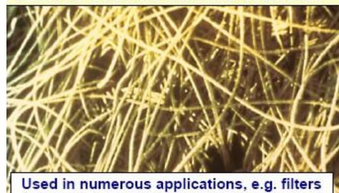
Used in numerous applications, e.g. filters or cushions for geomembrane protection
