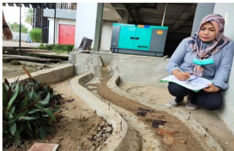
Figure 9. Placement of the 60^\circ crib slope angle
