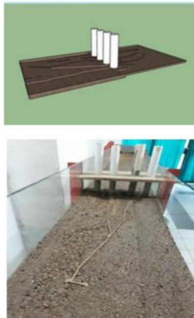
Figure 10. Sediment movement pattern during t = 30' .
