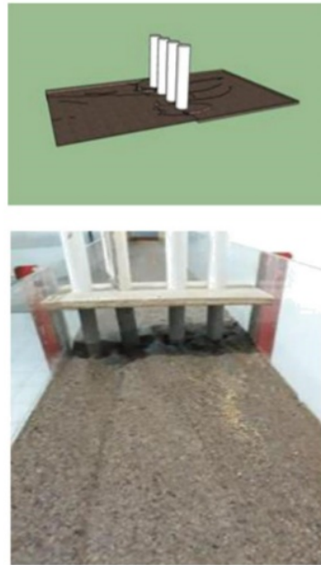
Figure 11. Sediment motion pattern during t = 60' .
