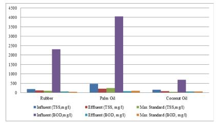
Fig. 1: Wastewater at influent-effluent of Gasing WWTP
