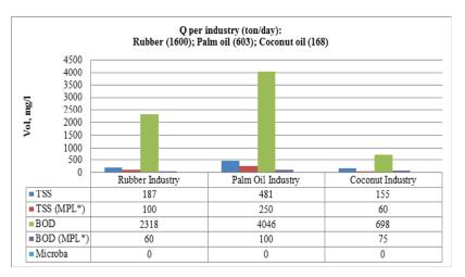
Fig. 2: Wastewater data at Gasing WWTP influent
