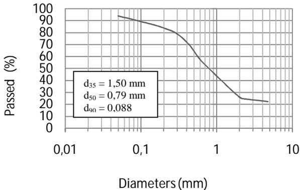
Fig 7. Grain size distribution in SPD canal
