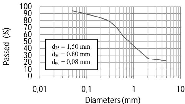
Fig 8. Grain size distribution in SDU canal
