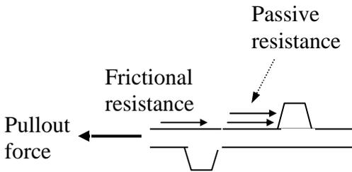
(b) Friction and passive resistance (pullout test)
