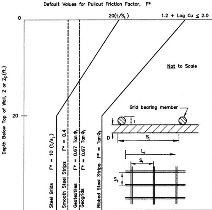
**Figure 6.6:** Pullout resistance factor for different types of reinforcement
