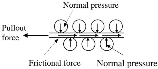
(a) Pure friction (Direct shear test)
