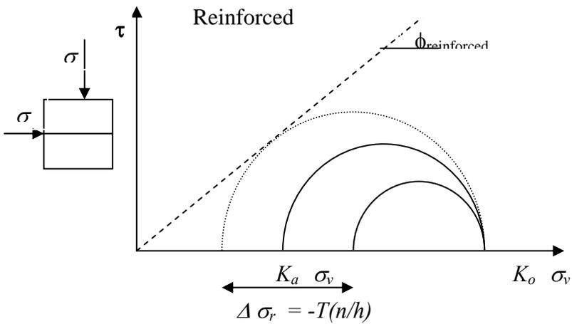
**Figure 6.8** Mohr circle for unreinforced and reinforced soil
