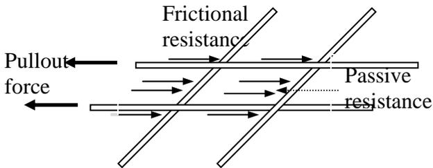
(c) Friction and passive resistance (pullout test)
