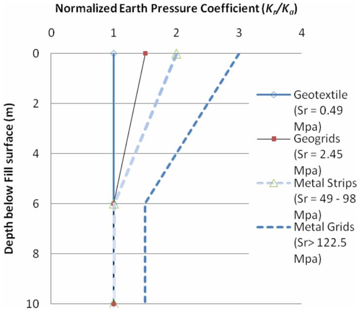
**Figure 6.7:** Relationship between  $K/K_a$  and the stiffness ratio for the design of reinforced soil structures subjected to body force
