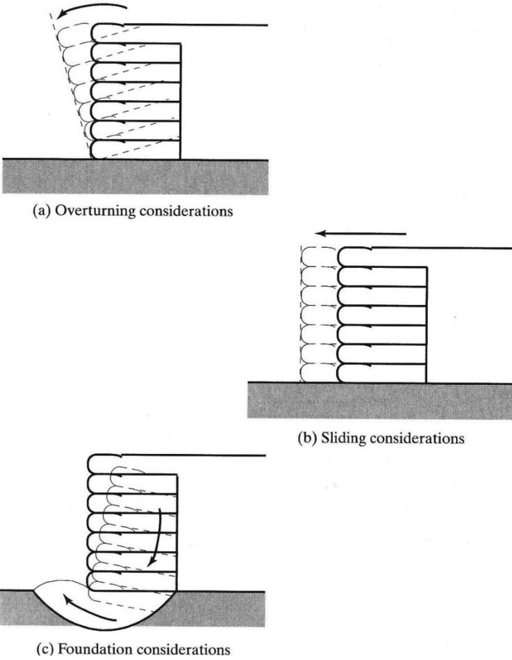
**Figure 6.3:** External failure mechanism in reinforced soil structures (after Koerner, 2005)
