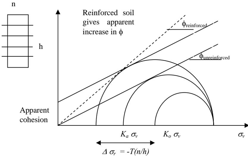
**Figure 6.1:** Basic mechanism of soil reinforcement and failure strength envelope (After Schosser and de Buhan, 1990)
