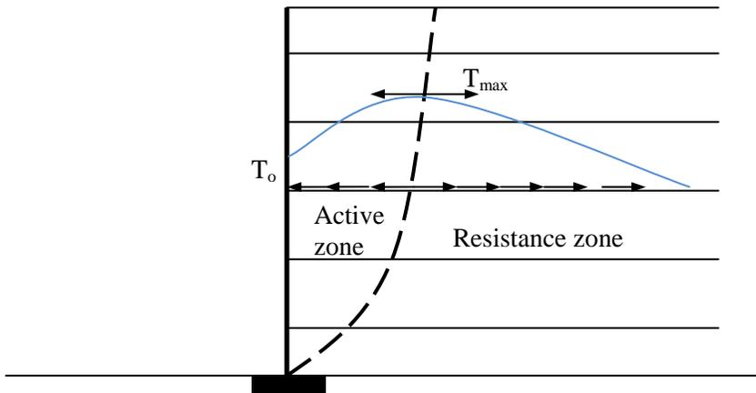
**Figure 6.4:** Location of critical slip plane or locust of maximum tensile force in reinforcement
