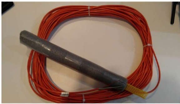
(a) Piezometer transducer
