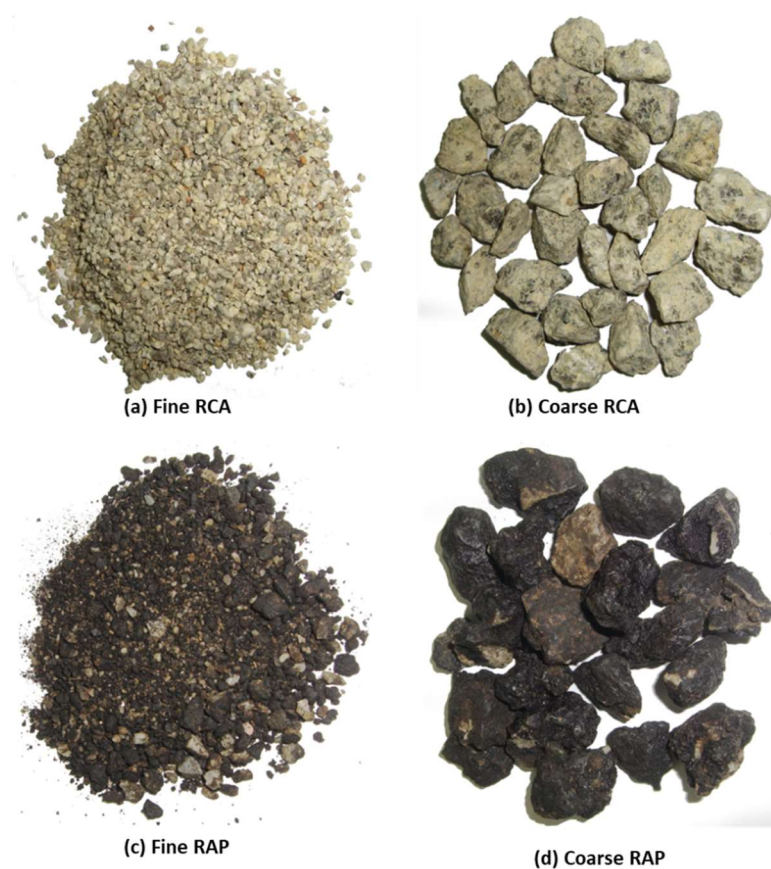
Figure 2. RCA and RAP used for construction of GBS at Pilot study site
