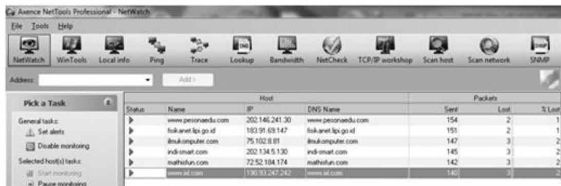
Gambar 6. Pengukuran Paket Loss di SMUN 04
