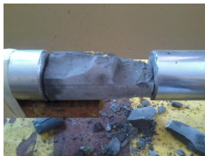
Figure 3: Failed control specimens after dynamic load impact
