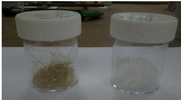
Figure1: Micro steel and polypropylene fibres
