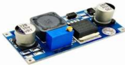
Gambar 4 Modul Regulator Stepdown
