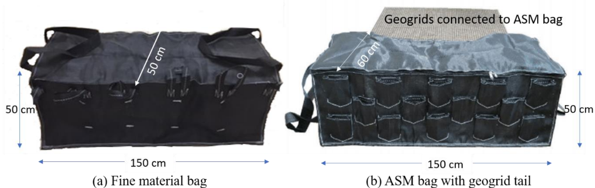
Figure 2. Geotextile bags for fine material and ASM.
