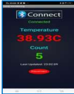
Gambar 15 Tampilan Aplikasi Sensor MLX90614 ( >37^{\circ}\text{C} )
