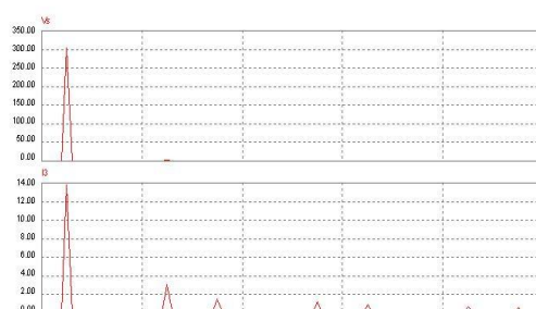
Gambar 2.2 Voltage and current waveform images of the net due to the use of nonlinear load
