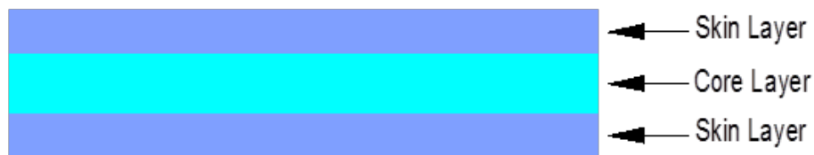
Figure 1: Sandwich Concrete Layers
