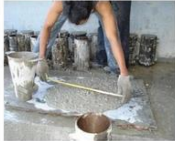
Beton SCC (slump flow)
